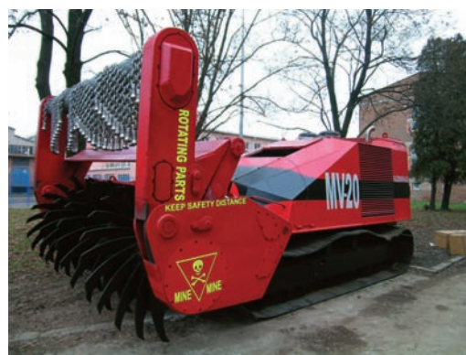
MV-20 Heavy Double Flail-Tiller Mine Clearing System Basic technical characteristics of MV-20
