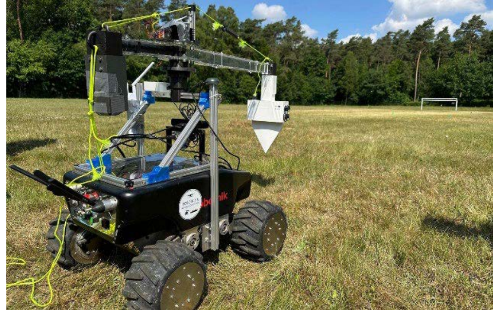
Robotnik Summit-XL + gprSense® during data collection at DOVO
