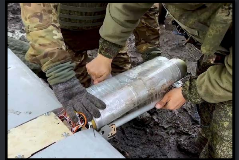
A Russian Molniya UAV equipped with thermobaric warheads from the Shmel rocket-propelled flamethrower. Photo from Russian media, February 2025
