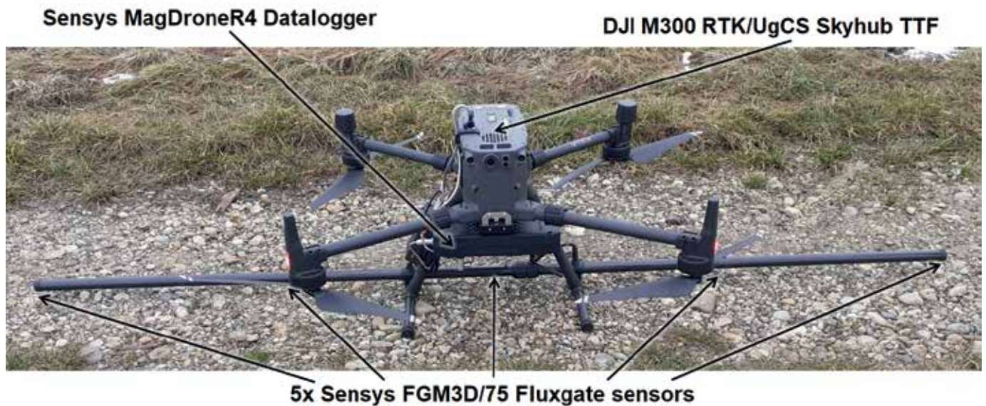
Figure 1 The compact setup of the Sensys MagDroneR4 magnetometer system
