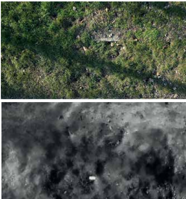
Figure 2. The image shows a land mine with a green metal casing placed on green grass. The top image represents the terrain as seen in the visible spectrum, while the bottom image shows the same terrain in the thermal spectrum.
