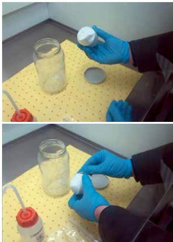
Figure 1 - Using preconcentrator at Swedish EOD and Demining Centre (SWEDEC) to swab objects for identification of objects with trace explosives contamination.
