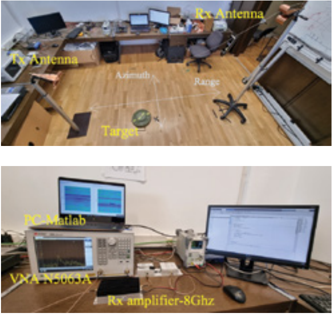
Figure 2. Experimental setup, with adjustable bistatic Rx and Tx antenna configuration, VNA and PC-Matlab .
