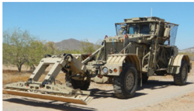
Figure 1. 3D GPR system from Kontur AS mounted on a mine detection vehicle
