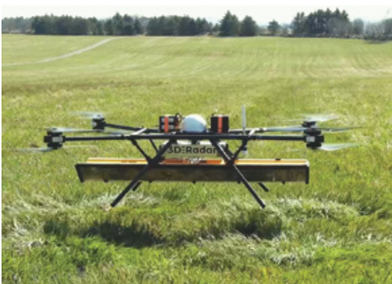
Figure 2. UAV 3D GPR system from Kontur AS during operation
