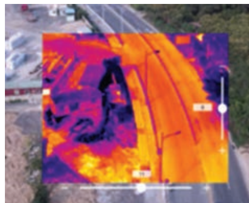
Figure 8. The visible wavelengths image and TIR image are fused in dual-sensor camera.
