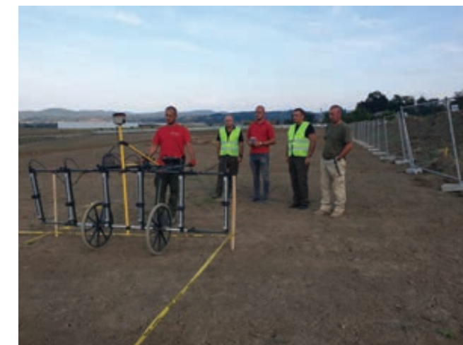
Photo 2: Use of devices that allow the application of a passive and active method on ERW clearance project related to Data Center construction site in Kragujevac
