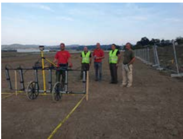
Photo 2: Use of devices that allow the application of a passive and active method on ERW clearance project related to Data Center construction site in Kragujevac
