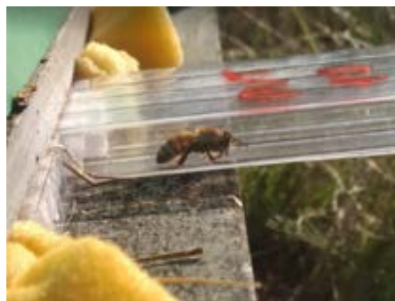
Figure 1 - Honey bee in cartridge tunnel containing a preconcentrator.
