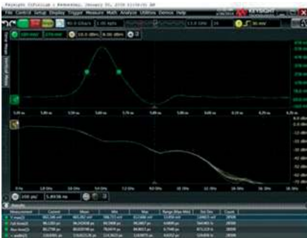
Fig. 8. Output pulse from generator captured by oscilloscope.
