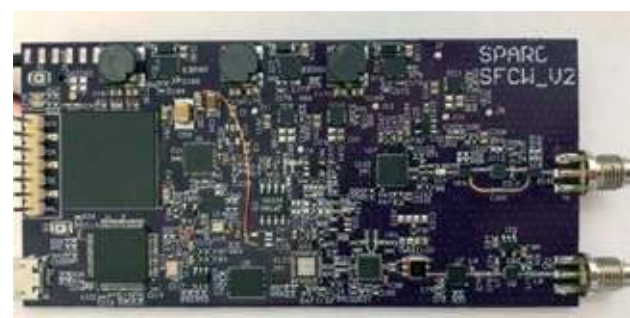
Fig. 5. Hardware realization of the Steeped Frequency Continuous Wave Radar.
