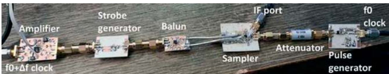
Fig. 10. Experimental set-up of generating and sampling UWB signals.
