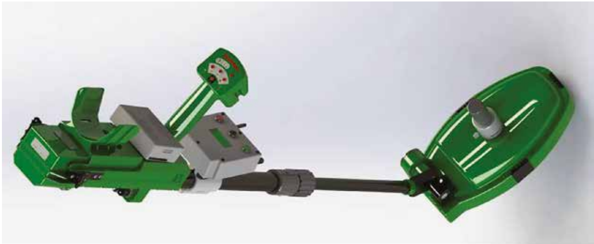
Figure 3 - Minehound VMR3 equipped with GNSS RTK head tracking
