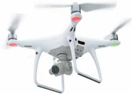
Figure 1: Shows a 1.4kg, DJI Phantom 4 Professional, mini-size quadcopter. Image credit www.dji.com .
