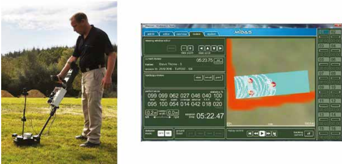
Figure 5 - MIDAS Outdoor Training System, Detector (Left) and Software (Right)
