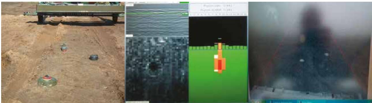
Fig. 2. Multispectral detection head and examples of antitank mine detection with different sensors (from left to right: GPR, MD, IR) of WITI's the multisensor mine and IED detection system
