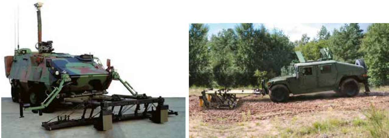
Fig. 3. Two examples of multisectional mine detector systems constructed in Military Institute of Engineer Technology for the Polish Army
