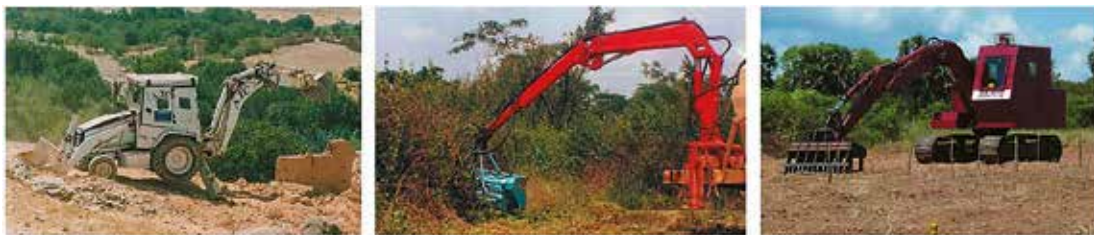
The pictures shows a backhoe in Afghanistan, an articulated hydraulic mulcher arm on the back of a Werewolf MPV in Angola and an Arjun 3 raking excavator in Sri Lanka.
