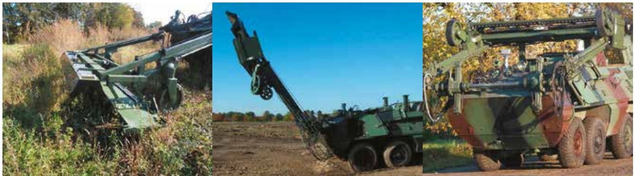
Fig. 1. Multisensor mine and IED detection system constructed in the Military Institute of Engineer Technology for the Polish Army
