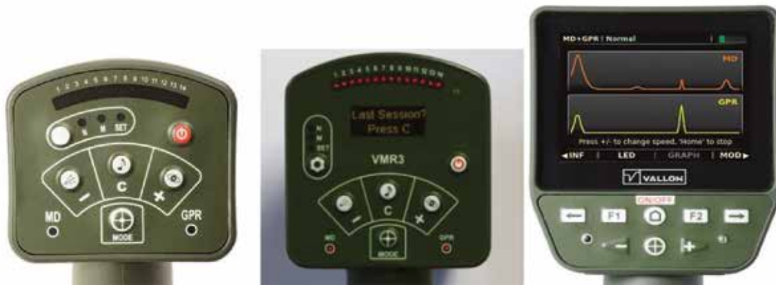
Figure 2 - Minehound Displays, LED (Left), Alphanumeric (Centre), Graphical (Right)
