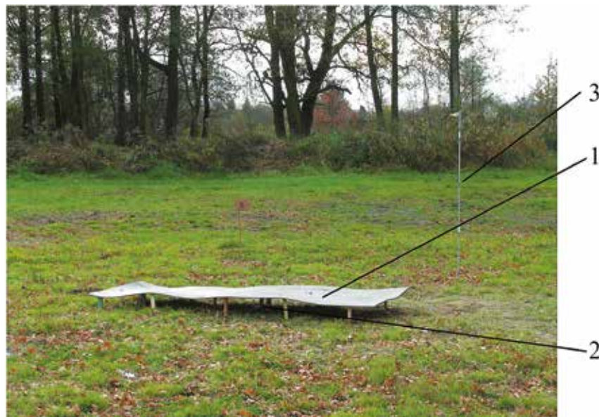
Fig. 4. Area where the impact of explosive charge explosion of the flexible armour was tested: 1 – flexible armour; 2 – explosive charge; 3 – height gauge
