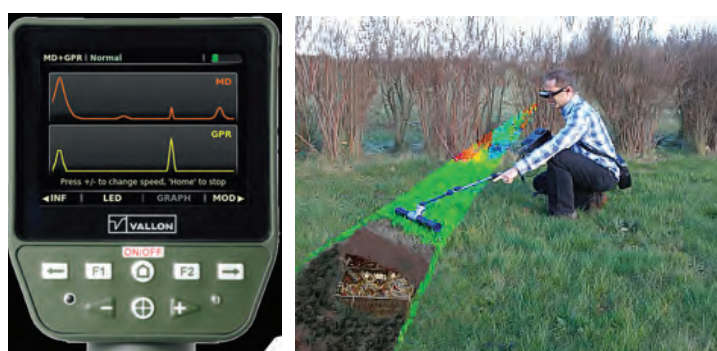
FIG. 4. Current HMI solutions for MD data. a) HMI of a Vallon VMR3G dual-sensor detector [4], b) next-generation metal detector for archaeological exploration utilizing eyewear for data visualization [13].
