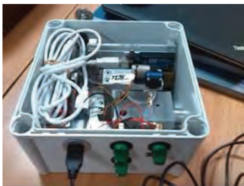
FIGURE 2: Prototype of the explosive vapour sensor (lid off)
