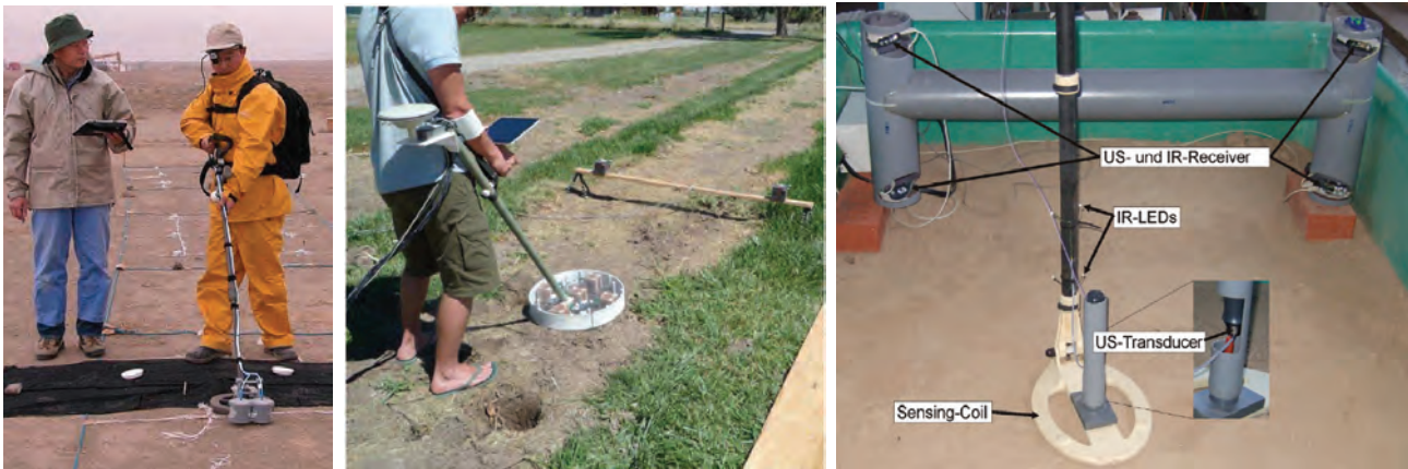
FIG. 3. Current solutions for a search head tracking system. a) optical system using CCD camera mounted on a search head [6], b) inductive system utilizing a transmitter coil as a magnetic beacon [2], c) ultrasonic-optic system [9].
