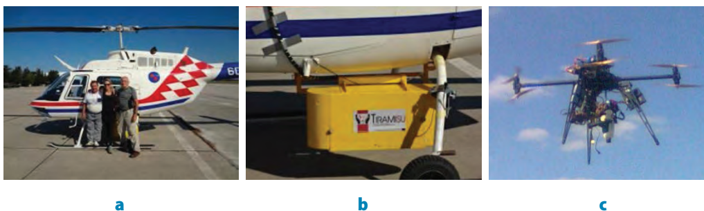
FIGURE 5. Final versions in 2015 of aerial platforms with hyperspectral sensors. a) team for hyperspectral survey from helicopter Bell-206B. b) The line scanner V9 and full frame UHD-185 are located inside of yellow pod on helicopter, c) multi engine UAV with UHD-185.
