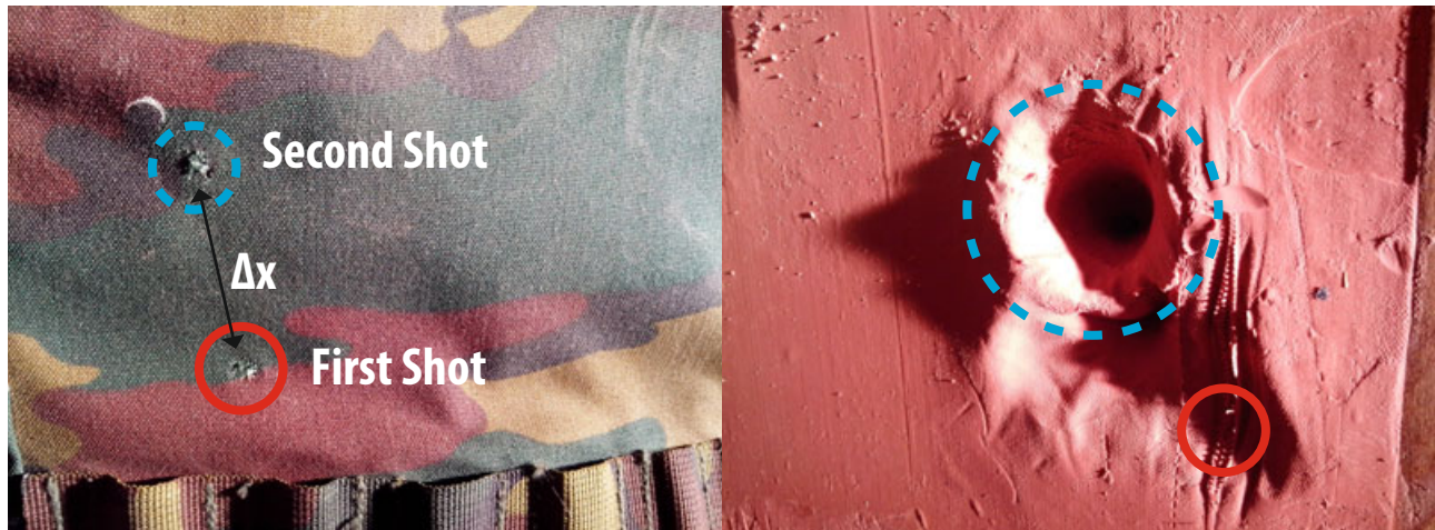
Fig.2 A double tap test resulting in perforation (of the second impact). The first impact point is circled with red and the second with dashed blue. Left: the fragmentation vest. Right: the plasticine backing.
