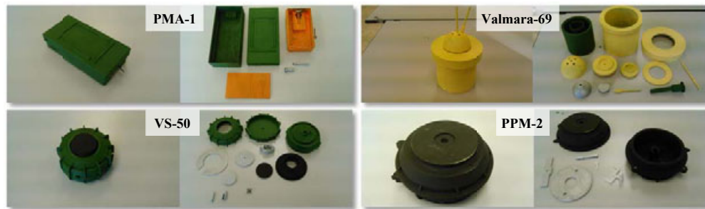
Figure 1. Surrogate antipersonnel landmines designed by CAR CSIC-UPM.
