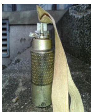
Fig.4: armoured fuze of KB-1 (the slider is outside the fuze)
