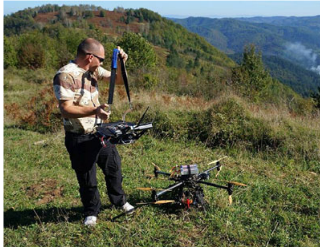
Figure 2. RPAS MRx8 and operator - preparation for aerial survey
