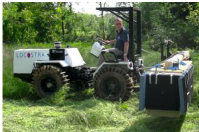
Figure 6. LOCOSTRA V2- LUCIFER GPR Array
