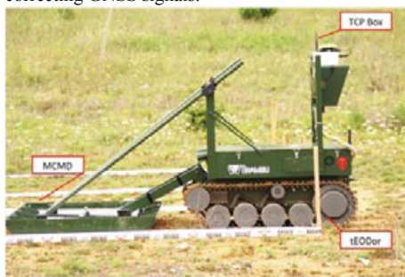
Figure 1 Teodor mobile robot platform with the MD and TCP box FIG3. TEODOR WITH MD AND TCPBOX
