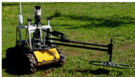
Figure 2. The Clearpath Husky mobile robot with the Vallon VMP3 metal detector.
