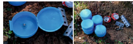
Figure 6. a) Metallic spheres as landmine simulants, b) landmine simulants and metallic clutter items.
