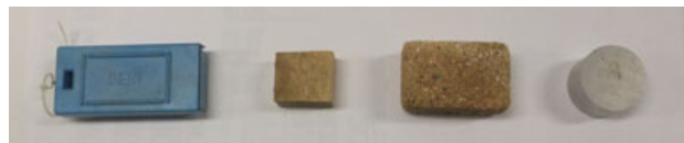
Fig. 1. Four targets for classification test: from left, landmine surrogate, wood, stone, aluminum.
