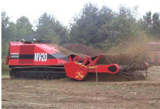
Photo 1: Demining machine, MV-20
