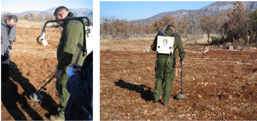
Figure 5. Hirvoje Stipetic and Nikola Gambiroza (CROMAC technical manager) QC after machine demining. The soil is plowed and many small rocks appear on the surface.
