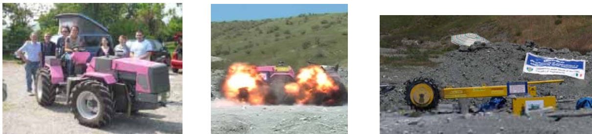
Fig. 2. Locostra: tractor with team on board, tractor during blast resistant wheels test and ballistic pendulum for pre test of blast resistant wheels.
