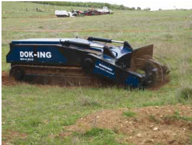
Fig. 4. a – Diesel demining machine with flail, b - Diesel - electric demining machine, c - Electric demining machine (5 t, MV-4 flail, options)
