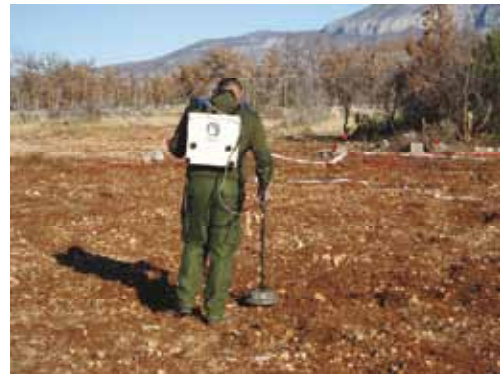
Figure 4. ALIS operated in machined demined area. The soil is very soft, because it was excavated, but we found the capability of GPR imaging by ALIS is not much affected.
