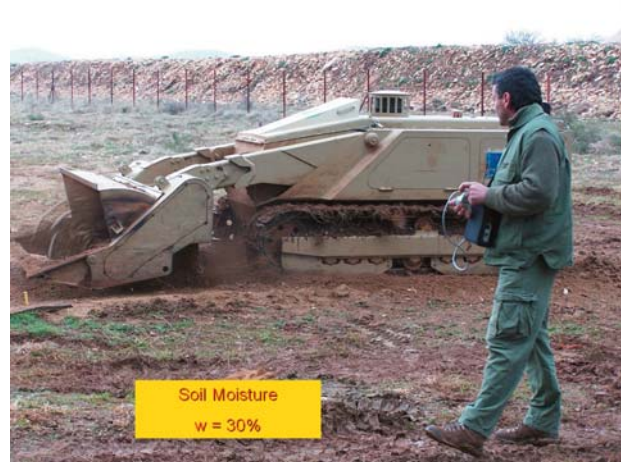
Fig.2. Forming of new loose layer of soil under the tracks
