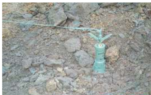
PROM-1 prepared for testing of "Mini MineWolf"
