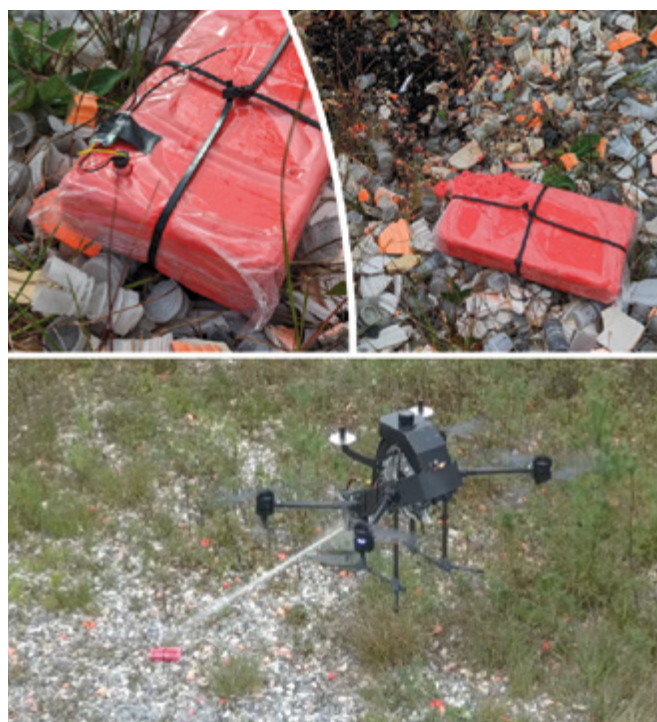
Figure 2: Neutralization of an inert C4 explosive charge by precise destruction of the detonator using a gel-water shot. 4 m stand-off distance, 2 cm accuracy, 4 min total operation time.
