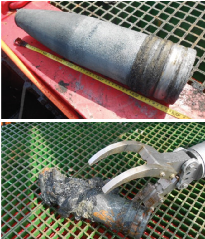
Figure 2: (Upper photo) A munition experiencing the effects of concretion before cleaning. (Down) The same munition after cleaning
