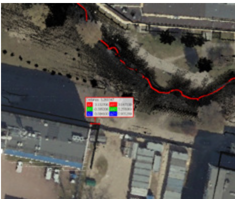
Figure 14: Measured error ( \Delta xy > 1.4m ) to ground truth (CP2 – see figure 10).
