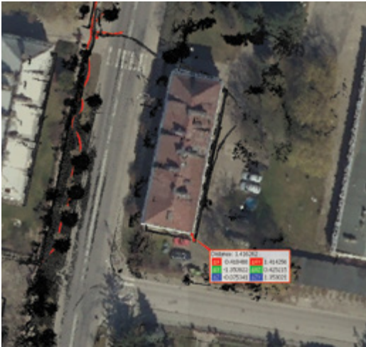
Figure 13: Measured error ( \Delta xy > 3m ) to ground truth (CP1 – see figure 10).
