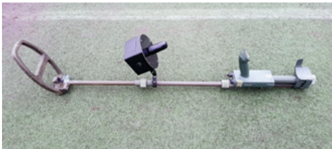
Figure 1. Tracker attached to metal detector.
