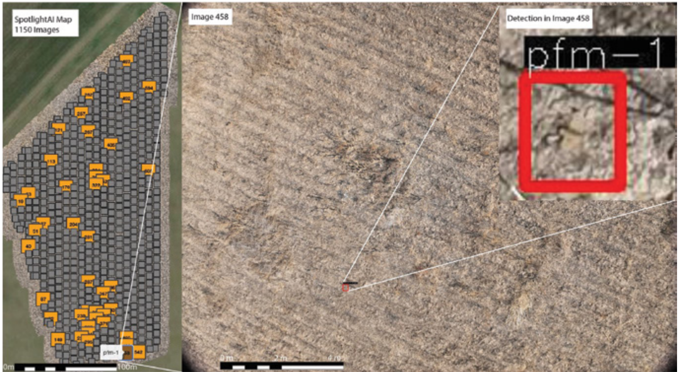
Figure 1. Example of real-world drone survey processed by SpotlightAI, with detection of a PFM-1.
