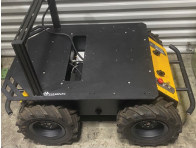
Figure 1: The Husky UGV Platform. The manipulator arm will be mounted on top of the robotic platform.
