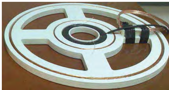
Figure 3. Laboratory prototype of a sensing head.
