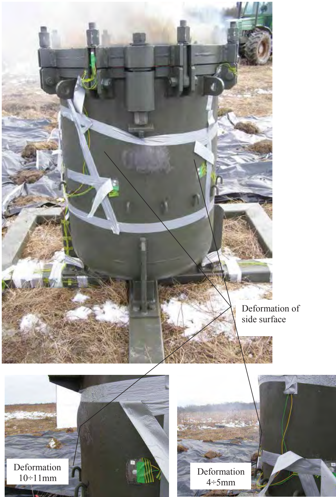
Fig. 10 Deformation of the container side surface-front view (top figure) and side view (bottom figure).
