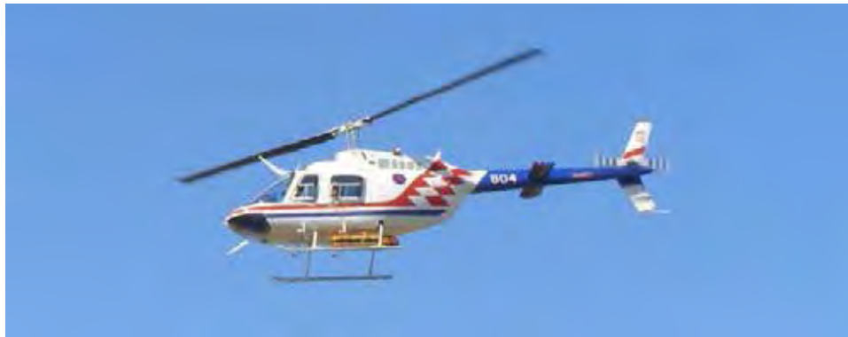
Figure 4. Helicopter Bell-206 with the T-LHSIS in the orange-black container installed under the helicopter.
