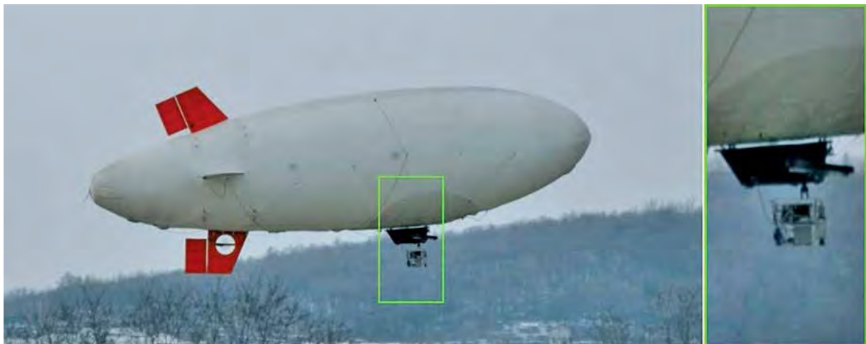
Figure 3. Blimp with T-LHSIS (in two green rectangles).
