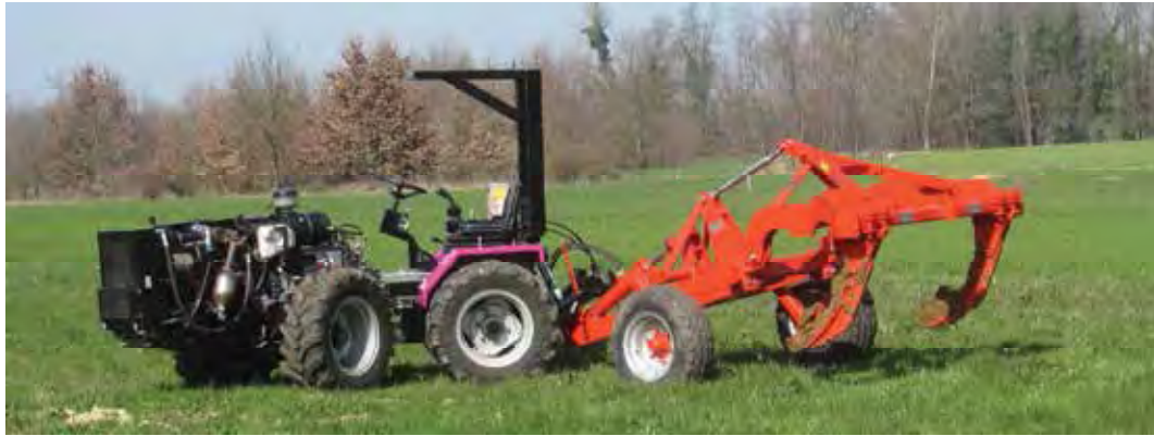
Fig.4. Mobility measurements in performance tests: measurement of minimum radius of curvature
