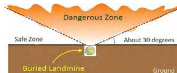
Fig. 1 Impact angle between prodder and terrain. It's possible to distinguish the dangerous zone from the safe one.
