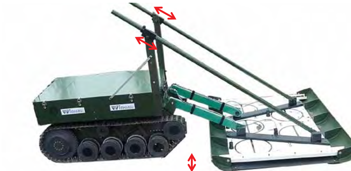
Figure 3 Mounting mechanism with the MCMD and the tEODor platform
