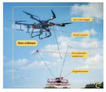
Figure 1. Illustration of MinesEye system
