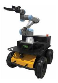
**Figure 2.** Mobile manipulator robot. It consists of a Husky A200 mobile platform, equipped with a UR5e robotic arm and a Robotiq 2F-85 gripper.
