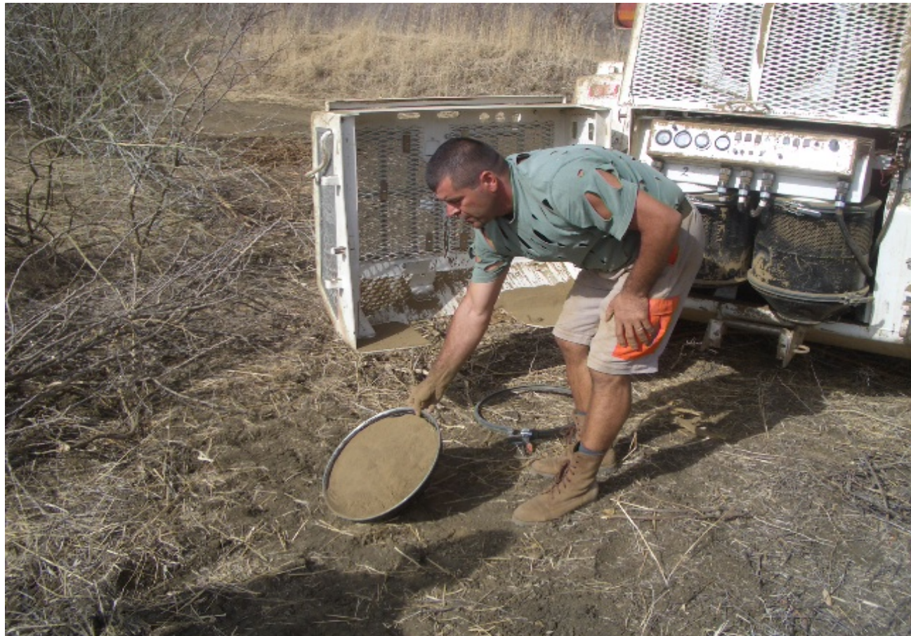
Photo 3: Machine undergoing hourly service; see the amount of dust in filters.
