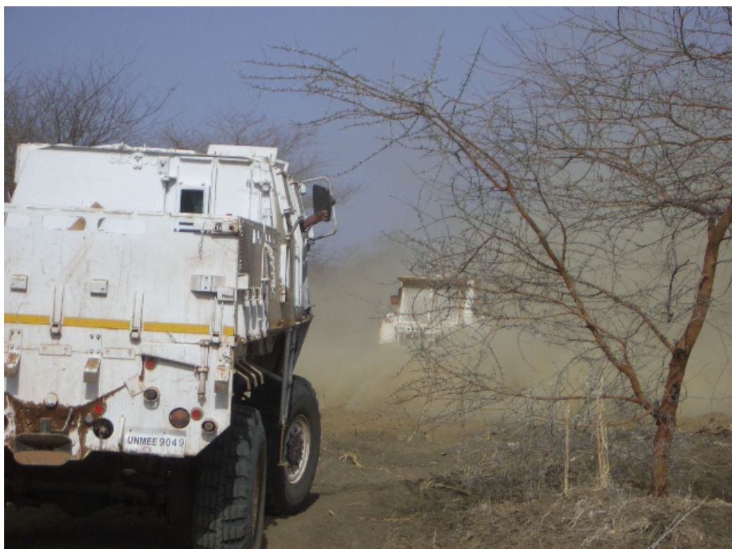
Photo's 6&7: Tapir MPV utilized as control vehicle for Bozena-4 mini flail.
