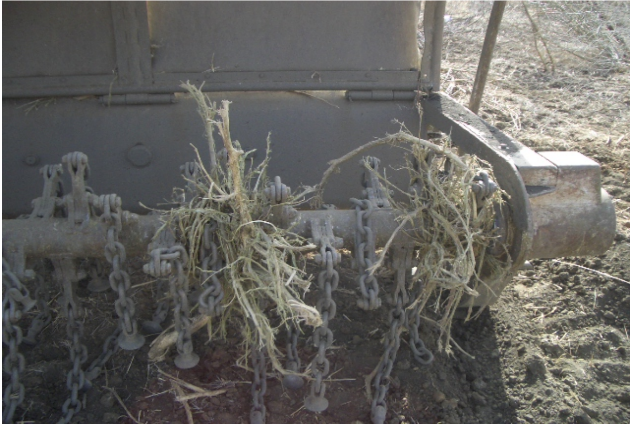
Photo 4: “Sekel” bush entangled on flail axle; had to be removed hourly or sooner.
